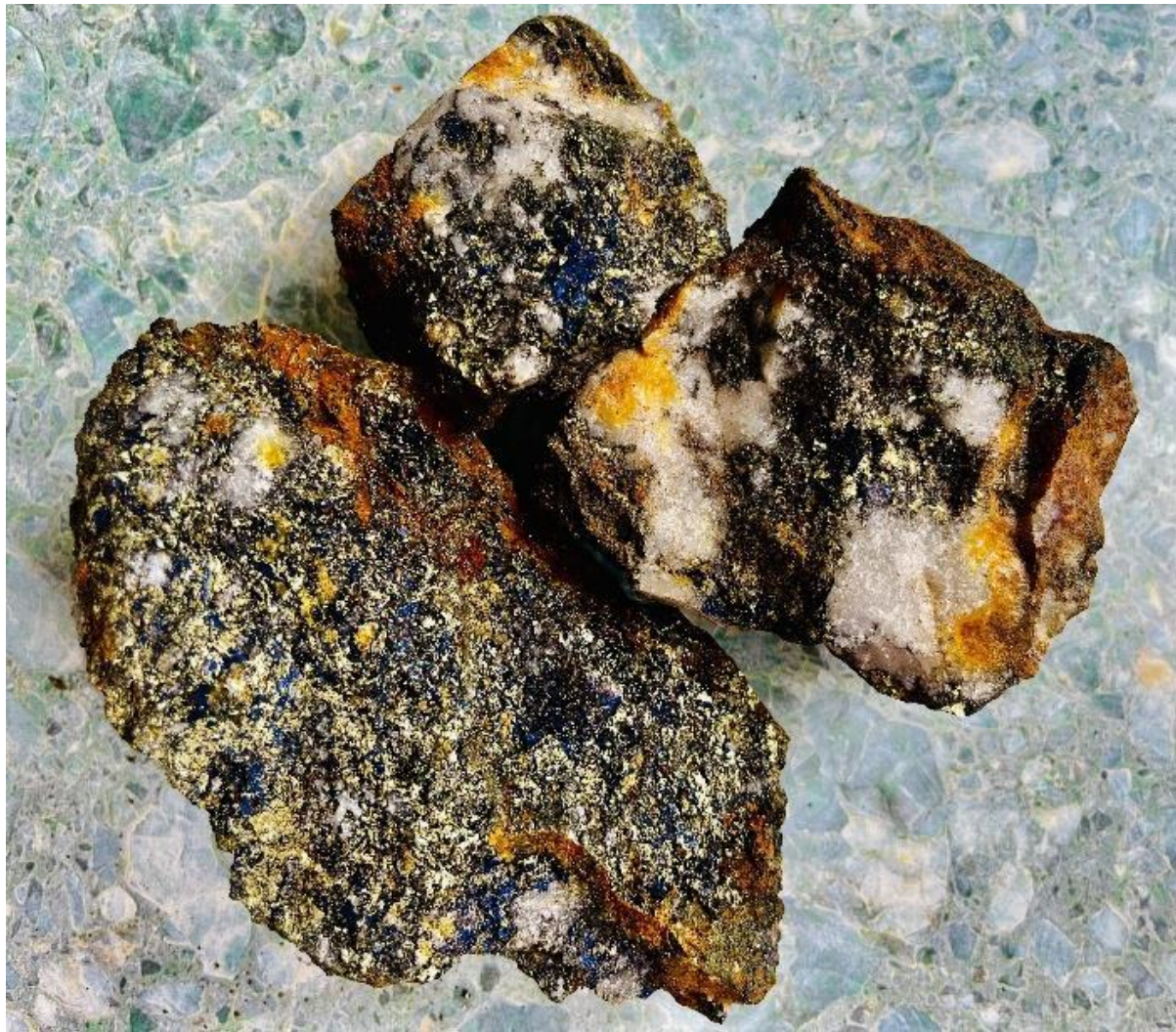
11.35% Cu, 0.17% Mo, 1.55 g/t Au, and 129 g/t Ag in sample A0284675 with coarse chalcopyrite, bornite, and molybdenite
